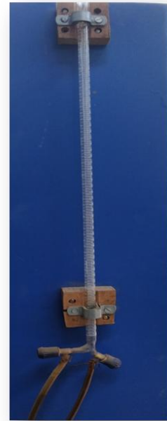
Figure 2 Measurement panel & fuel consumption measurement burette
